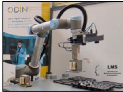
Manipulation of transformer for oven assembly at LMS premises
